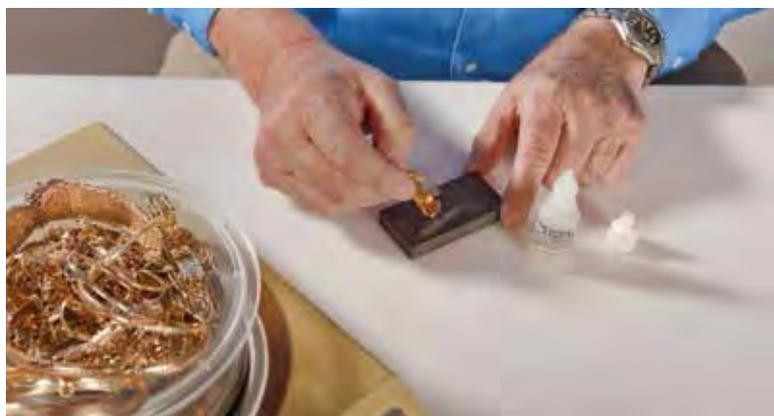
sample in strong acids, the gold content can be accurately determined. Base metals and other impurities are left behind in this process.
